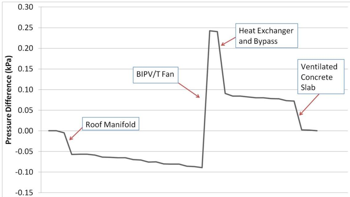
Figure 6: Pressure losses in the duct system for the1 estimated worst-case
