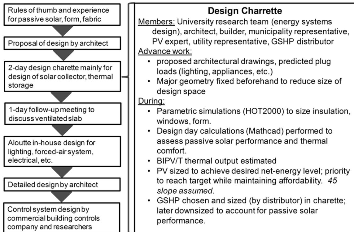
Figure 3: Design process outline for ÉcoTerra
