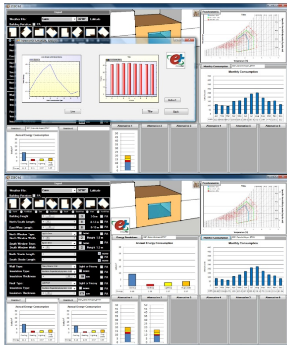
Figure 5a, Reference model and output plots including sensitivity analysis results.5b, model and output plots for design alternatives comparison.
